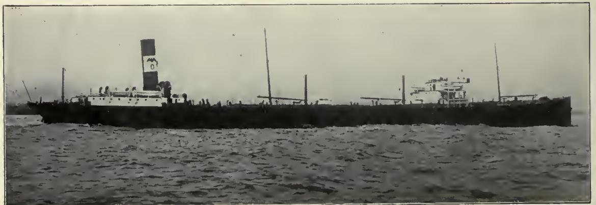
Tank Steamer "SAN HILARIO," Capacity 15,700 Tons. One of the fleet of vessels owned by the Mexican Eagle Oil Company, Limited, engaged in transportation of bulk oil.
